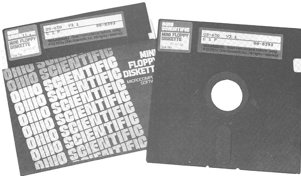
Figure 9: Typical Mini Floppy, Also Called Disk or Diskette. Note the White Write Protect Tab on the Right Edge (These may also be black). Any Attempt to Write Data or Save a Program on This Disk Will Fail and Yield an Error #4 Message.
