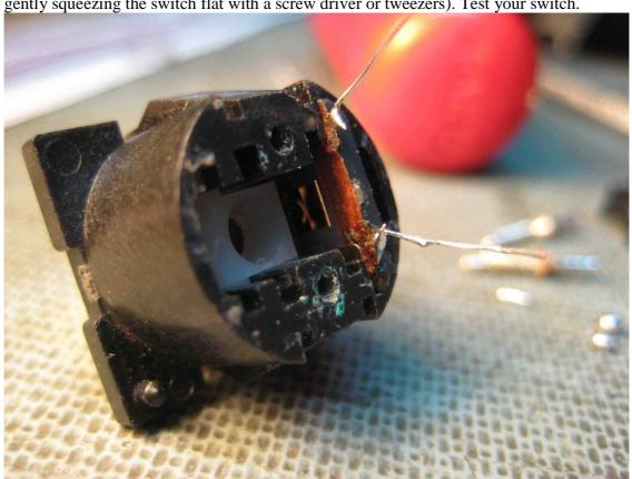
Tuck the new leads into the pin holes for terminal connection.
