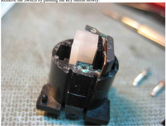
Here, the switch is out. You are seeing the spring metal actuator, not the contacts.
