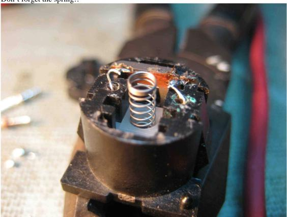
Now, replace the end cap, "screw your terminals" back into place while holding everything together tight. Test your switch and solder it back in place.
