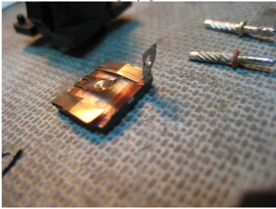
Here are the contacts. I've soldered new leads (30awg Wire Wrap)
