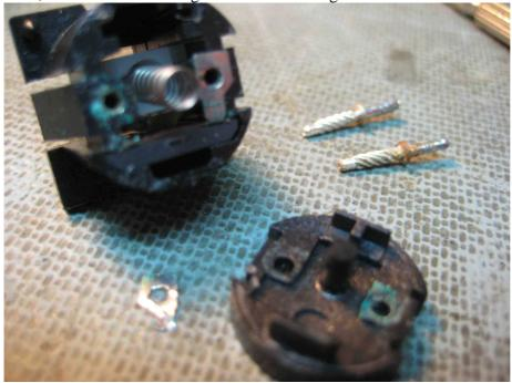
Zoom in for closer examination. See the switch lead broken on the left side? It's remains are right there on the bench below, ½ in the photo shot. No points for photography here!
