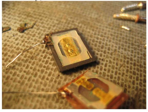
After sandwiching the switch, be sure it gets flat again (melt the solder quickly while gently squeezing the switch flat with a screw driver or tweezers). Test your switch.
