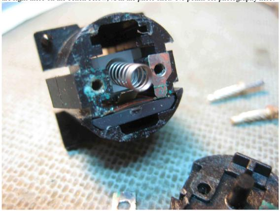
Remove the Switch by pushing the key button slowly.
