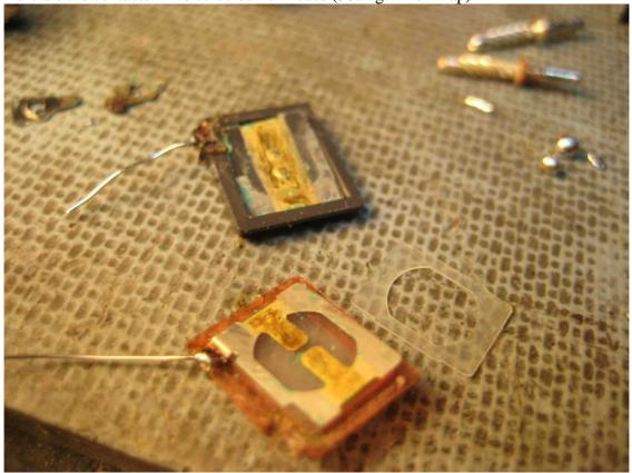
Carefully replace the insulator (which was removed to clean the contacts and solder new wires without melting it).
