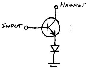
Since TTL gates can only source about .8 ma in the high state, Darlington transistors are required. I used GE type D40C4 rated at 6 watts, 0.5 amps, 40 volts, with a gain of 10,000. The diode is a 1 amp 50 piv rectifier. It serves to protect the transistor from the counter emf generated by the magnet coil. Note - for 48 volt magnets, use a D42D3 transistor with a 1 amp 100 piv diode.
