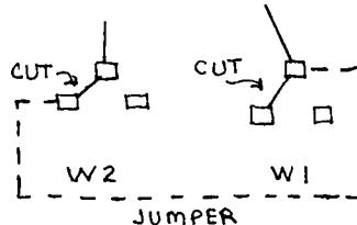
This converts Pin 21 on the 2716 EPROM from 02 clock to +5 volts. I suspect a similar change is required on BASIC 3 as well. Until I made these changes, my Cl required a "warm-up" period of 5 to 10 minutes. Now, it "boots up" at once.
