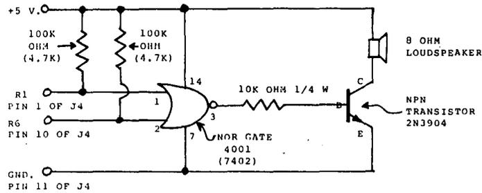
NOTE: Resistor values for 7402 IC are shown in parenthesis.
