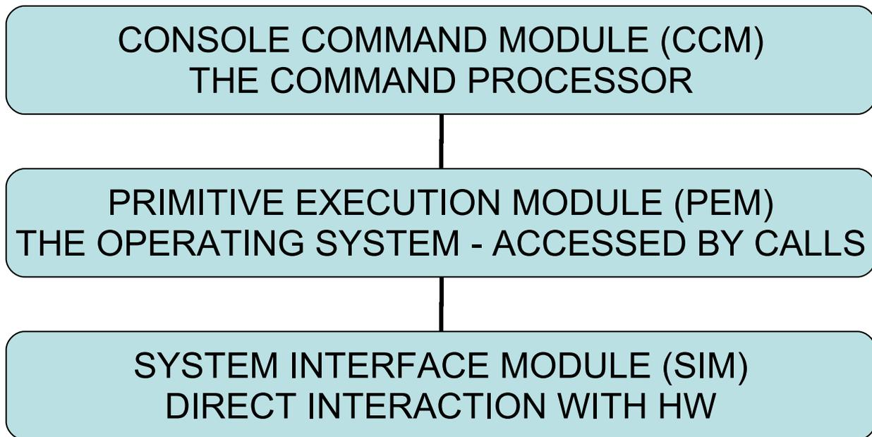
As the figure indicates, the layers of DOS/65 are strongly related to both the degree of host independence and the ease of use of that layer by the programmer. Each layer is described below.
