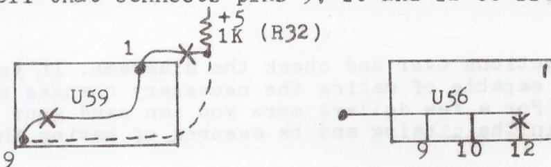
Replace U59 and U56 using sockets. Cut foil on U59 between pin 1 and the 1K resistor. Put a jumper between the 1K resistor and pin 9 on the foil side. Also hook a jumper from the 1K resistor to pin 1 of U60.
