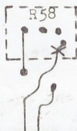
Underneath the R58 5K variable resistor cut where marked. This will isolate pin 9 of U65.
