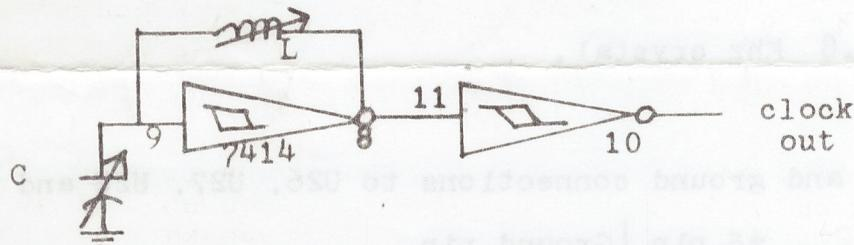
This oscillator circuit should be stable within  $\pm 2\%$  which should give a stable display.
